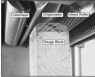
Figure 21. Location of chip breaker assembly.
